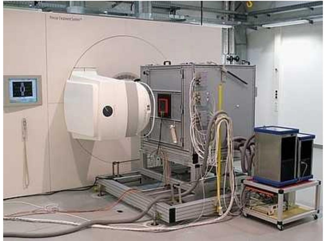
$$1 \text{ Gy} \rightarrow \Delta T = 0.24 \text{ m}^\circ\text{K}$$
